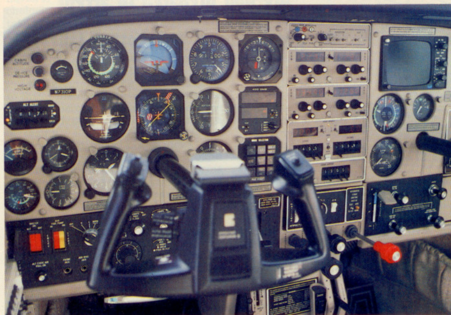
The extent of instrumentation on this single is measured by the array on its panel. Besides full avionics, an RDR-160 weather radar fits in at right. Fuel gauges are moved to the base of the center pedestal.
