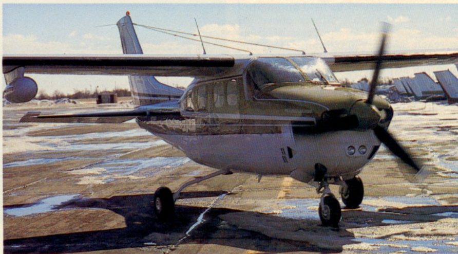
The P210 can carry a ramp weight of up to 4,016 pounds out to the run-up area. A pod housing the radar antenna hangs from the right wing.
