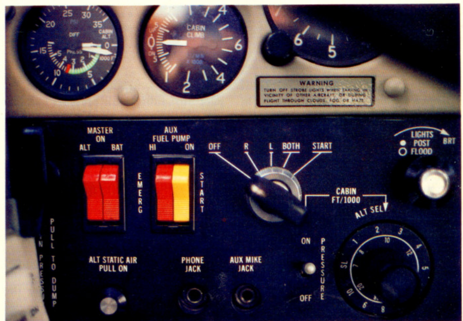
Cabin altitude and pressure differential are shown on the instrument at left, while climb or descent of the cabin is seen on the other instrument. Pressure selection is done with the knob at lower right, which shows 2,300 feet as the desired cabin altitude.
