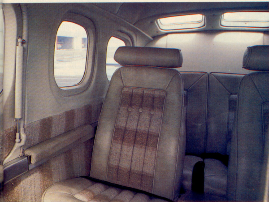
Porthole-like windows are required for better cabin-sealing capability, but reduce all-around visibility. The half-sized emergency exit on the plane's starboard side at lower left.
